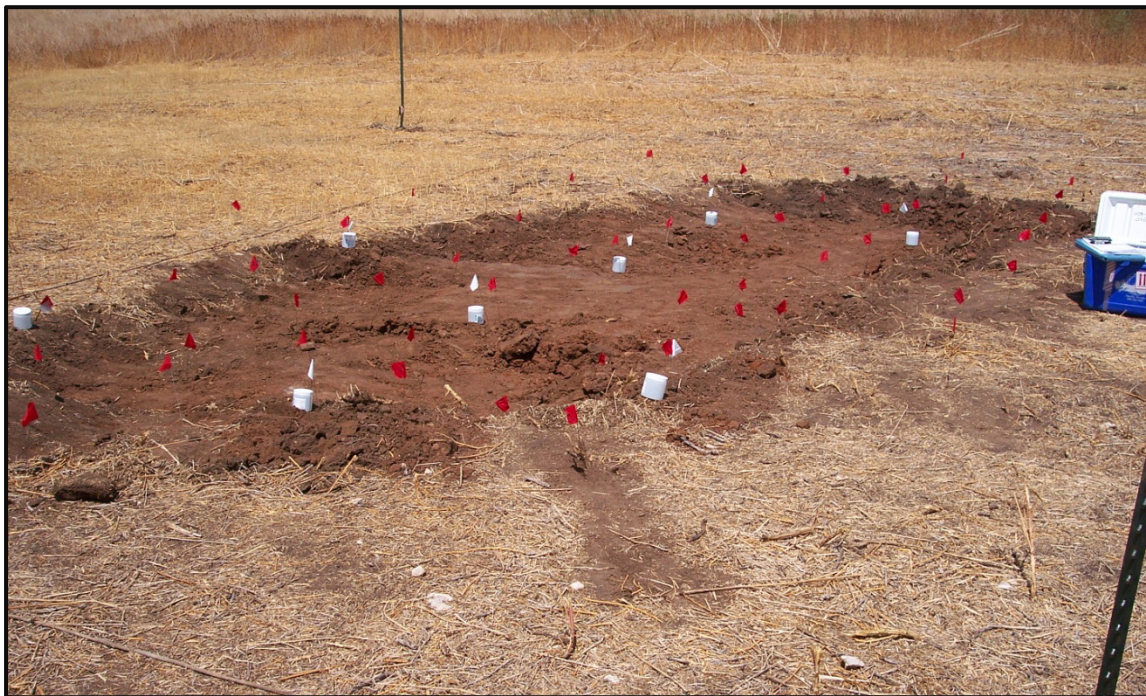
Figure A-18. Post Removal Action Soil Sampling Locations and Preparation for AOI #1. [Red Wire Flags Correspond to Post-Excavation FIDLER Measurement Locations & White Flags and White Sample Containers are at Soil Sampling Locations].
