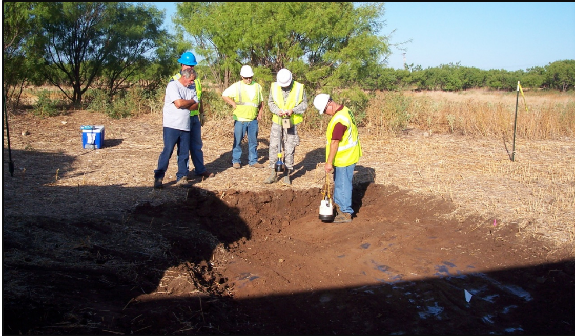
Figure A-10. FIDLER Scanning of Excavated Area in AOI #1 (View to West).
